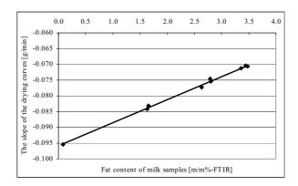
Figure 4 The slope of the section (between 40 and 90 minutes) of dehydration curves as a function of fat content of skimmed milk samples.
