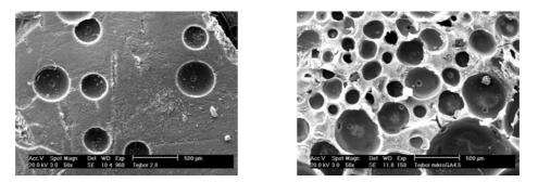
**Figure 6** Scanning electron microscopic images of milk skins of a 2.8% (left) and a 3.6% (right) fat content skimmed milk samples. Magnification: 50×.
