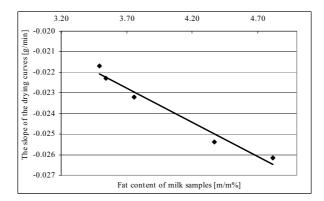
Figure 5 The slope of the section (between 75 and 120 minutes) of dehydration curves as a function of fat content of skimmed milk samples.
