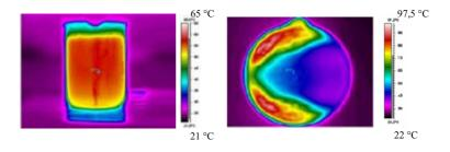
Figure 1 Infrared images of microwave heated distilled water (left) and ketchup (right).
