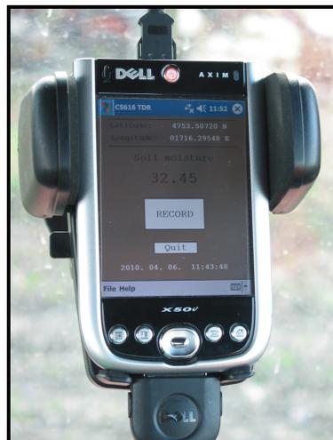
Figure 6. The software running on the PDA recording the soil moisture content
