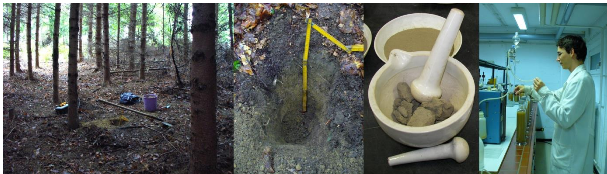
Figure 3.9. Surface soil sampling in the Farkas Valley (1-2), pounding the soil samples (3) and analysis of particle size distribution using Köhn pipette (4)
