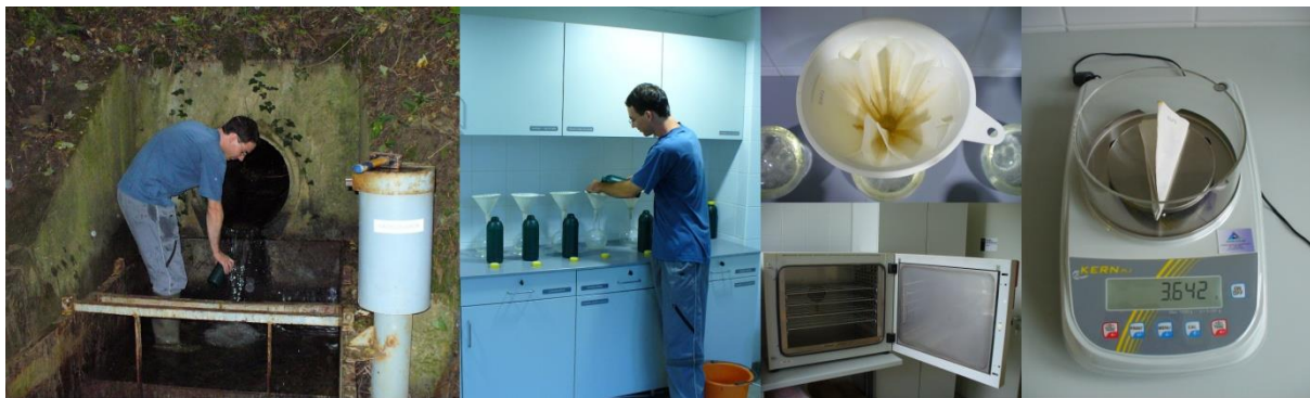
Figure 3.6. The process of gathering SSC data: water sampling (1), filtering (2-3), drying (3) and weighing (4) of the filter papers
