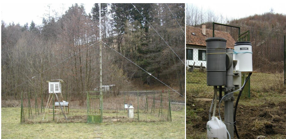
Figure 3.3. The central meteorological station (left) and the tipping bucket rain gauges (right; white: “ c l ”, gray: “ h hm ”) in front of the main research building in the Hidegvíz Valley
