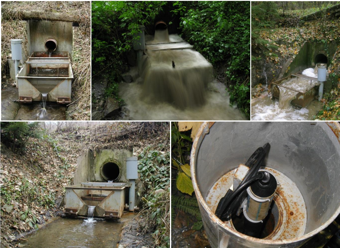
Figure 3.4. Stream gauging station at the outlet of the Farkas Valley (1: low flow; 2: high flow) and the Vadkan Valley (3: high flow; 4: low flow; 5: data logger)
