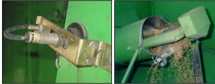
Figure 3.2 1.1. Yield and grain moisture sensors built in the harvester
