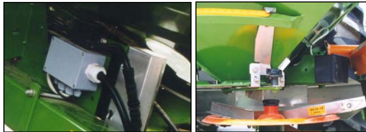
Figure 3.3.1.3. The job computer and the electric double shutter system on the disc spreader
