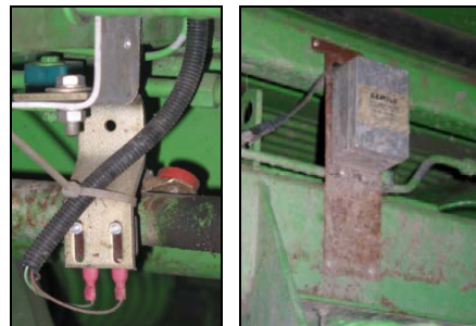
Figure 3.2.1.2. The speedometer and the inclinometer
